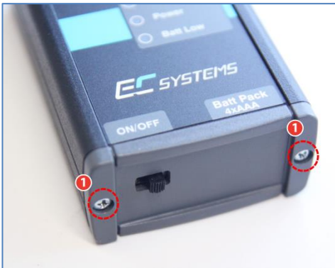
Figure 2 » View of the screws allowing access to the battery compartment.
