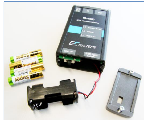
Figure 3 » View of the removed battery container
